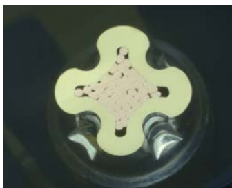
Figure V-4: Micro-section of a defective sample, wire cross-section too small
