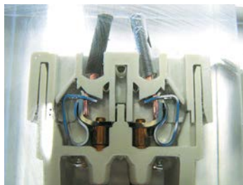
Figure VI-5: Termination with stripped stranded wire
