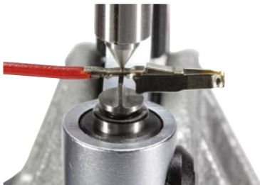
Figure V-11: Detail view of a crimp contact between the measuring tips
