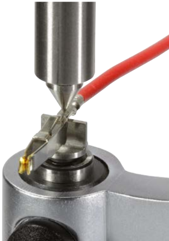
Figure V-10: Detail view of crimp contact
