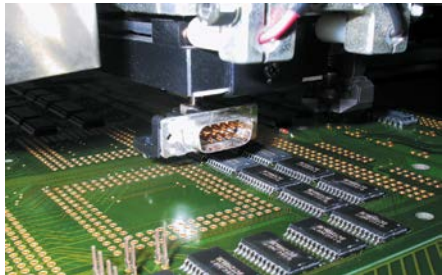
Figure IX-5: Pick-and-place machine with vacuum pipette and D-Sub
