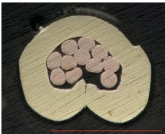
Figure V-7: Micro-section of a defective sample, wire cross-section too small
