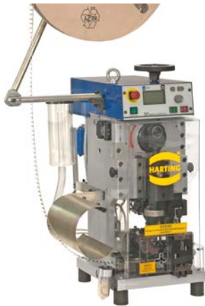
Figure V-18: TYPE BK crimping machine (fully automatic machine)
