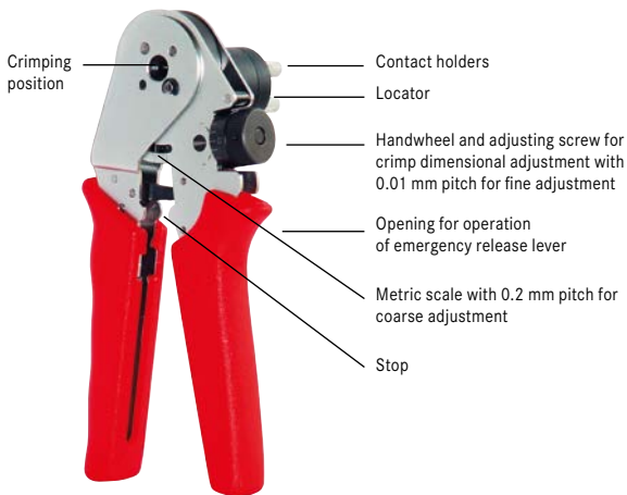
Figure XIII-16: Four-indent crimping tool
